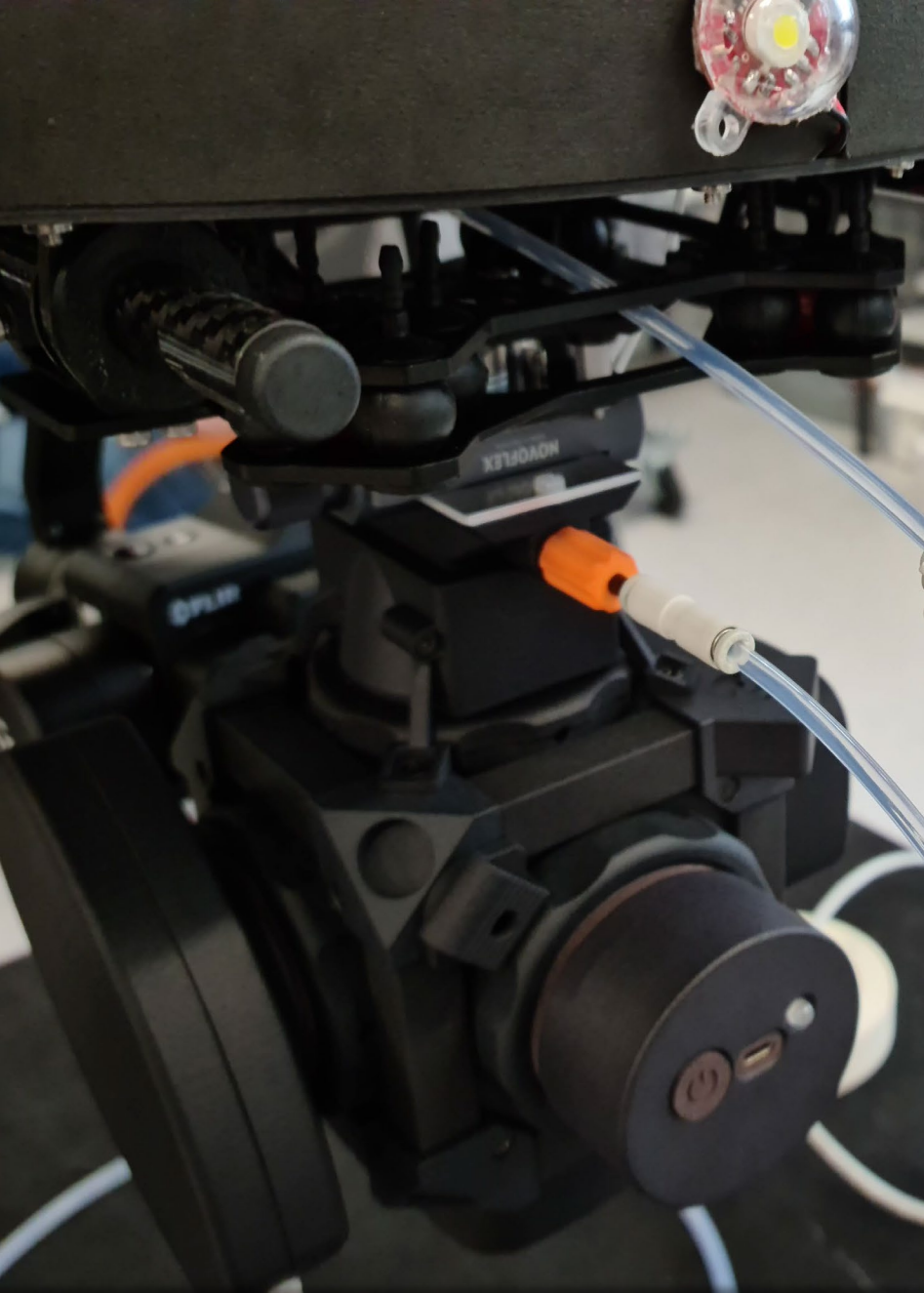
The Nuaer sniffer mounted on the Staaker BG-200
