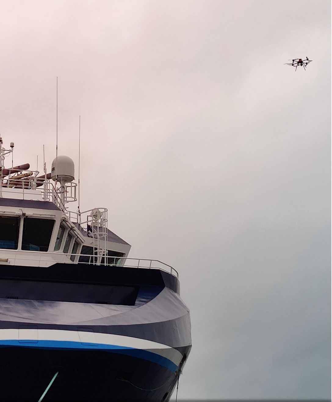
The Staaker BG-200 conducting emission monitoring with Nuaer sensor
