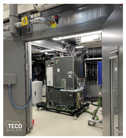
TECO 2030 Fuel Cell Module 400kW, FCM400: The unit is on the test bed at AVL's facility in Graz, Austria.
