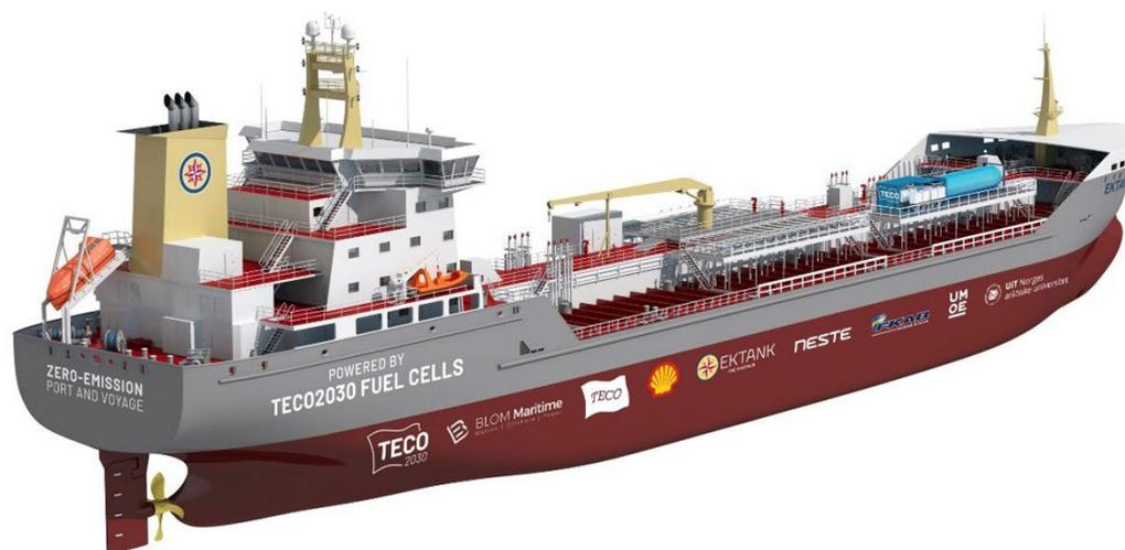
The HyEkoTank project will retrofit an 18.600 DWT product tanker with a 2.4 MW fuel cell system by TECO 2030 and 4000 kg compressed hydrogen storage for demonstration in 2024.
