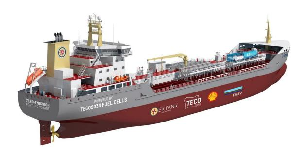
Picture text: Proposed Concept Hy-Ekotank. Retrofit installation of fuel cells with compressed or liquid hydrogen storage on existing Ektank vessels. The solution will eliminate emissions in port and reduce up to 100% of GHG emissions on voyages.
