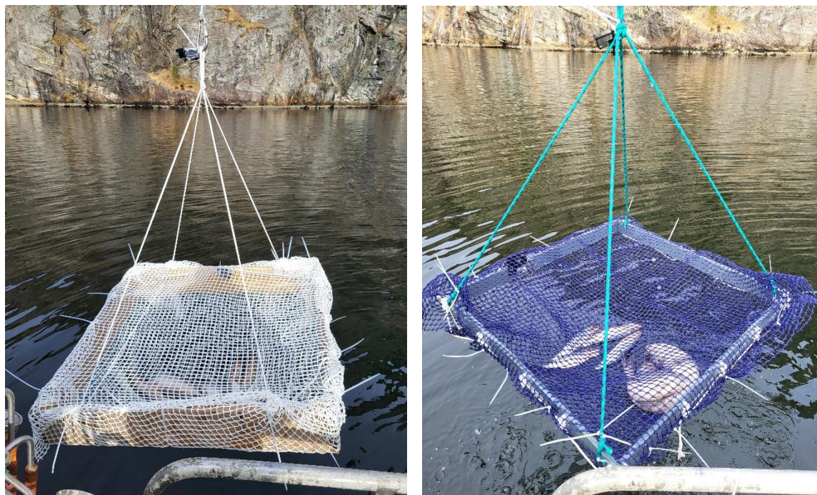
Figure 19 Deployment of rig showing two different netting material: white nylon net and blue SAPHIRE CFR net. A top mounted GoPro camera is visible here.
