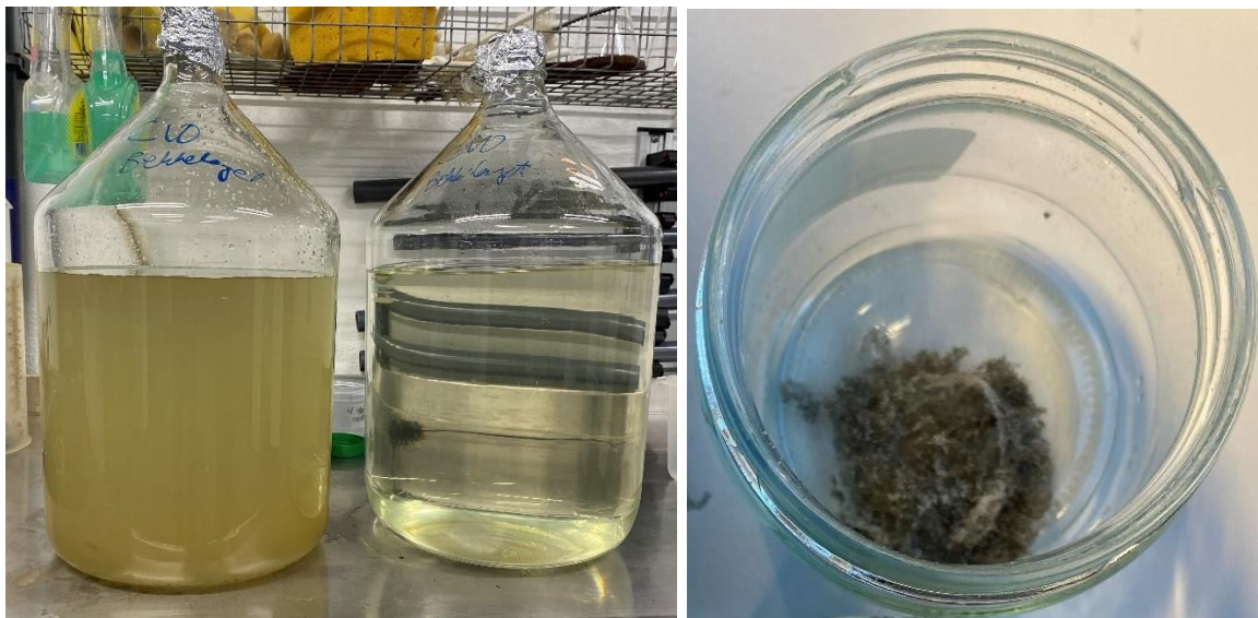
Figure 2: Photo of water samples collected (left) following low quality treatment (dark coloured) and high-quality treatment (light coloured) and particles isolated from the water phase (right). Photos: NIVA/Christian Vogelsang.
